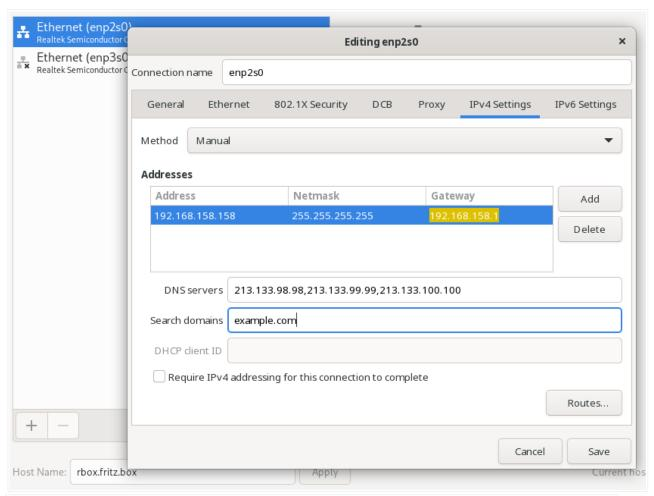
Fill out the form as shown in the example above. Unlike the usual information, you must enter 255.255.255.255 or /32 as the network mask in order to configure a peer-to-peer connection. The gateway information is displayed when you hover over the IP address in the Hetzner server management Web interface.
