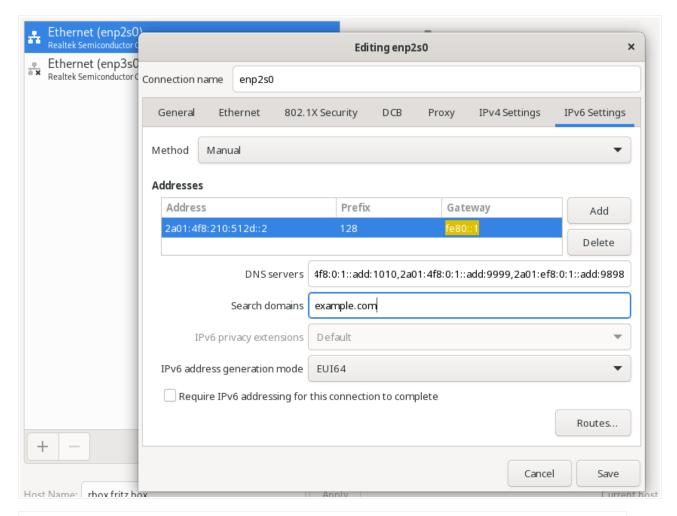
Again, fill out the form as shown in the example above. The IPv6 gagteway address is always fe80::1, the host address is ::2 appended to your network address. As prefix length enter 128 if you plan to install virtual maschines, otherwise use the well known 64.
